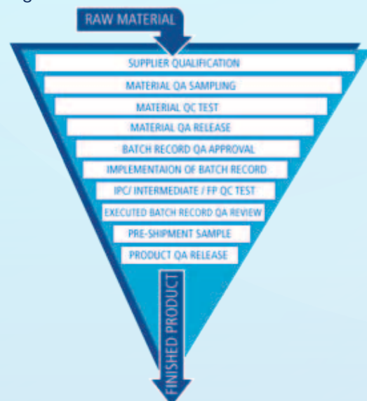
Figure 1. A top-down illustration of the Quality Control program in place in both our US and China facilities
